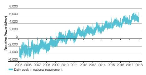
As you can see, the requirement for Reactive Power absorption has consistently increased for the last 10 years and our forecasts show this will continue. Figure 2.4 below shows how the need for Reactive Power generation has evolved over time, and shows the seasonal variation.
